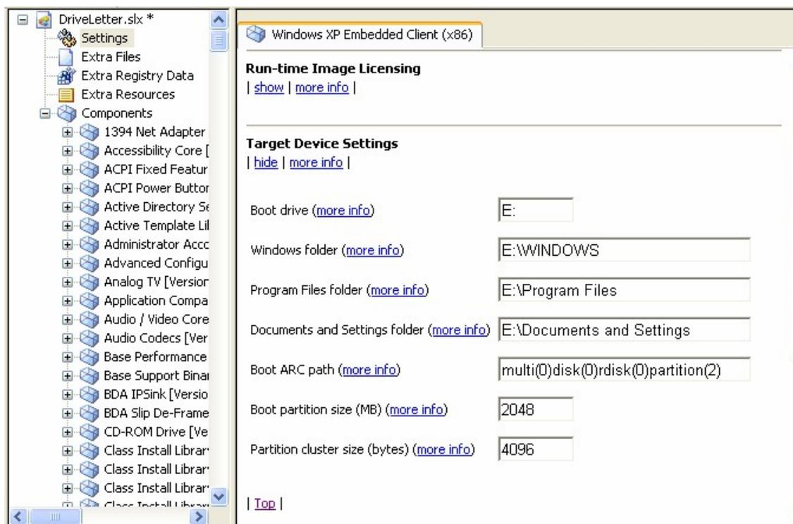
Fig 1 Target Device Settings – Is the drive letter correct?
